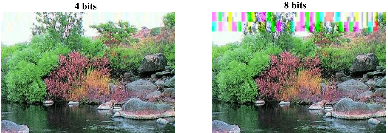
Figure 5: changing several bits in the first AC coefficient in a 90% quality image
