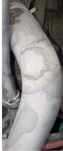
Figure 6. False positive case of an unflawed pipe.
