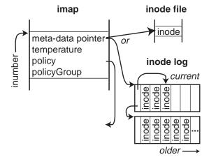
Figure 1. Meta data: the imap, inode logs, and the inode file.
