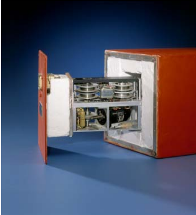
Figure 2. Flight Data Recorder's storage device
