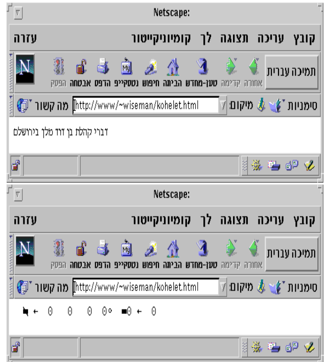
Figure 1.1: Results of displaying a Hebrew document with different fonts, using a Hebrew version of Netscape [12]. The top one provides the correct decoding of the letters. The second font does not define any glyphs for the higher 128 codes, so the browser displays some special graphical symbols.
