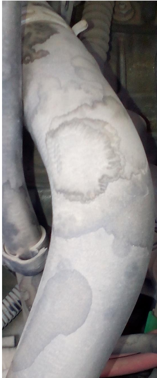
Figure 6. False positive case of an unflawed pipe
