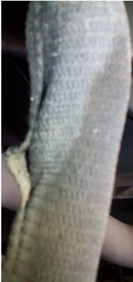
Figure 4. Example of a torn pipe
