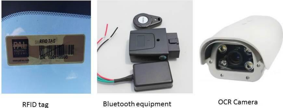
Figure 1. The three techniques used to identify vehicles - RFID tag on a vehicle, Bluetooth equipment and OCR Camera.
