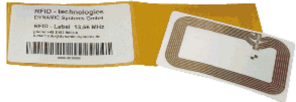
Fig. 1. Sticker of a 13.56 MHz RFID tag circuit and a bar code.
