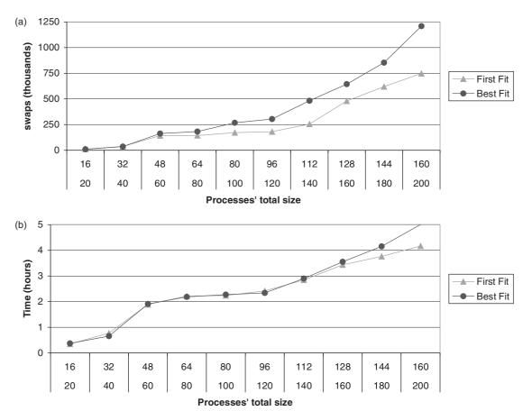
FIGURE 6. (a) Number of swaps using Best-Fit or First-Fit. (b) Execution time using Best-Fit or First-Fit.
