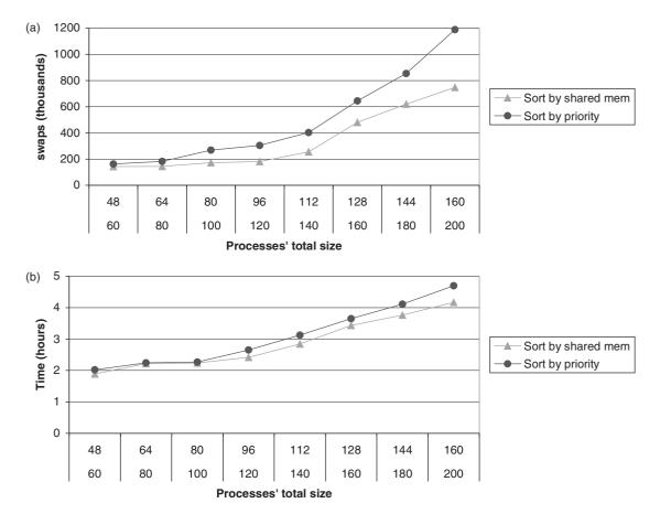
FIGURE 8. (a) SYNSHARED's number of swaps with different sorting methods. (b) SYNSHARED's execution time with different sorting methods.
