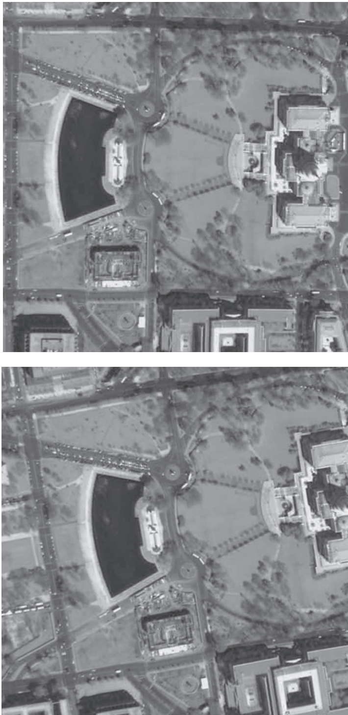
Figure 1.1. A reference image and its transformed image, extracted from an IKONOS scene acquired over Washington, DC. See Plate 1 in color plates section. (IKONOS satellite imagery courtesy of GeoEye. Copyright 2009. All rights reserved.)
