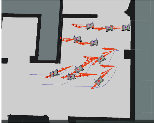
Figure 6: Simulated SAR Environment. The robots are represented in gray in the center of the screen, the black lines represent the structure walls and the red arrows and blue lines indicate the robots' planned trajectories. Note that this is not the user interface but only the simulation.
