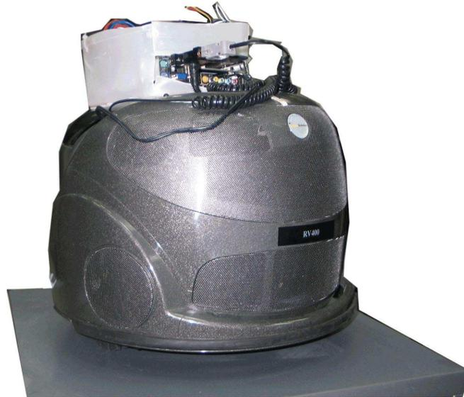
Figure 8.1: The RV-400 vacuum cleaner robot, with our lab’s computer overriding its commercial control software.
