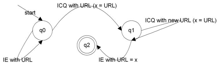
**Fig. 2.** Augmented DFA for recognizing the user receiving a URL in an ICQ message and then browsing it.
