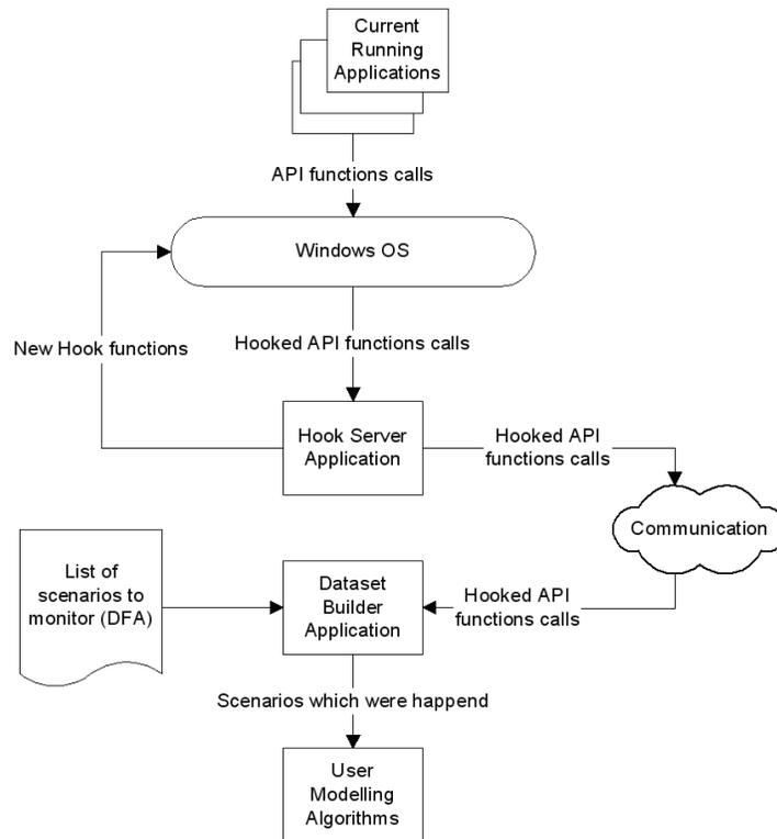
**Fig. 1.** Architecture of infrastructure for tracking actions across multiple applications.
