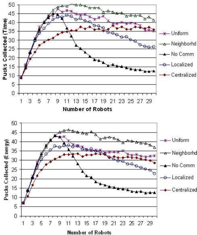
Figure 4: Comparing Adaptive Communication Methods based on Time and Energy Costs to Static Methods
