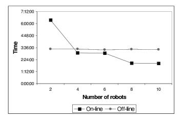
Figure 6.5: Coverage time of worst-case positions. Off-line results are calculated based on empiricallymeasured average velocity.
