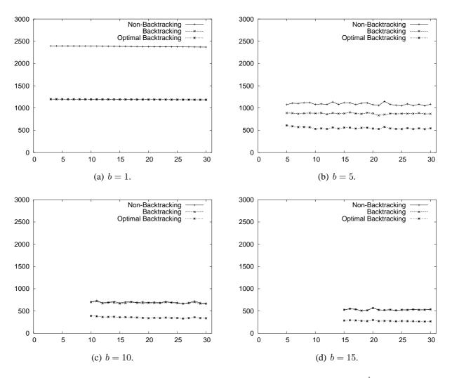
Figure 6.2: Coverage runtime when robots operate from *b* bases. Each base holds  $\frac{k}{b}$  robots. Each data point is an average of 100 trials
