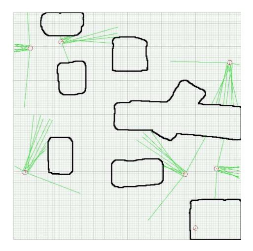
Figure 6.3: Simulation screen shot of six robots covering an outdoor environment
