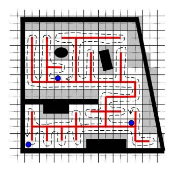
Figure 3.1: The grid, the spanning tree and the paths for three robots.
