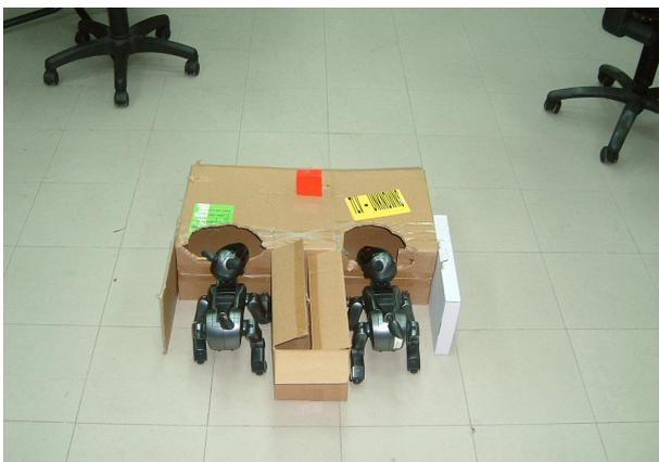
Fig. 1. Cooperative pushing (line formation) by AIBO robots.
