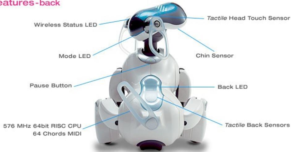
**Figure 9. Aibo front and back features.**
