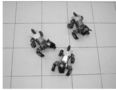
(b) Failure to maintain triangle formation. The top left robot has gotten too close.
