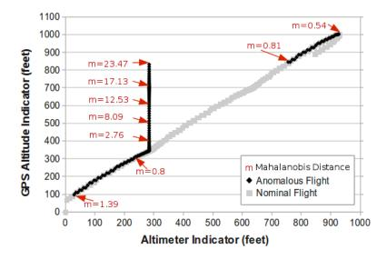
Figure 3.2: Example of Mahalanobis Distance as an Anomaly Detector
