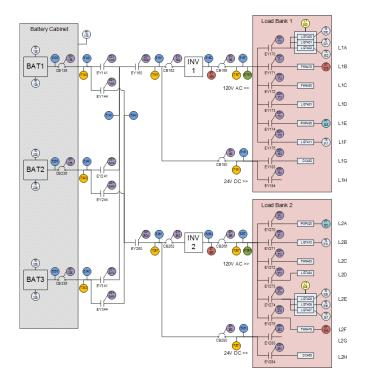
Figure 6.3: The Electrical Power System diagram.
