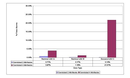
Figure 4.9: False alarm rates when applying the Mahalanobis distance on two and four correlated attributes.
