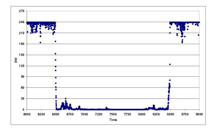
Figure 4.3: Constant UAV D: Mahalanobis distance (in std units) as a function of flight time (1/100 of a minute).
