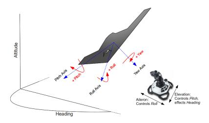
Figure 3.4: The *Heading* is affected by the *Elevation*
