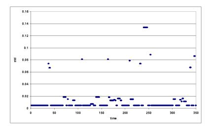
Figure 4.6: Direction Deviation UGV: Mahalanobis distance (in std units) as a function of movement time (1/10 of a second).
