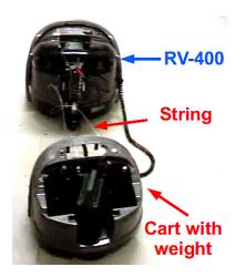
Figure 6.1: RV-400 tangled with a string connected to a heavy cart.
