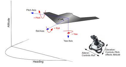
Figure 3.3: The Altitude is affected by the Elevation
