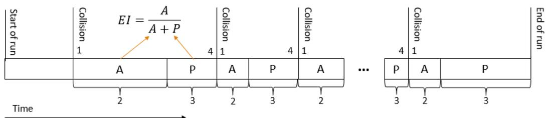
**Figure 2.2: Task life cycle from the perspective of an EI learning coordinating robot.**
