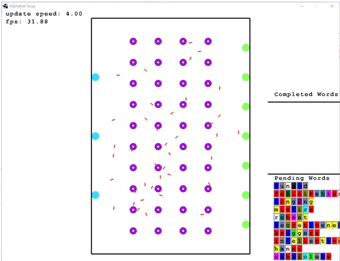
**Figure 5.1: The Alphabet Soup simulator. Red lines are the robots, Purple circles are the buckets, Green circles are the word stations and cyan circles are the letter stations.**
