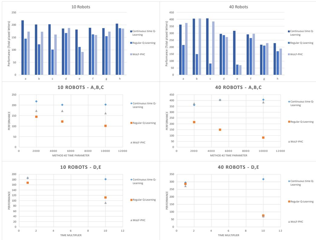
**Figure 5.22: Performance of the Minimum Over Actions approximation for regular Q-Learning, continuous time Q-Learning and WoLF-PHC, each with density quartiles as a state space.**
