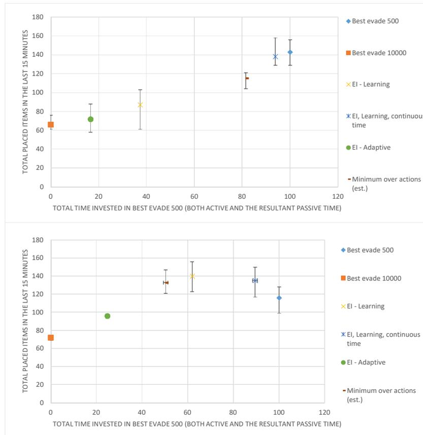
**Figure 5.9: Different variants of learning vs EI-based adaptation in Krembots for group sizes of 4 (upper chart) and 8 (lower chart).**
