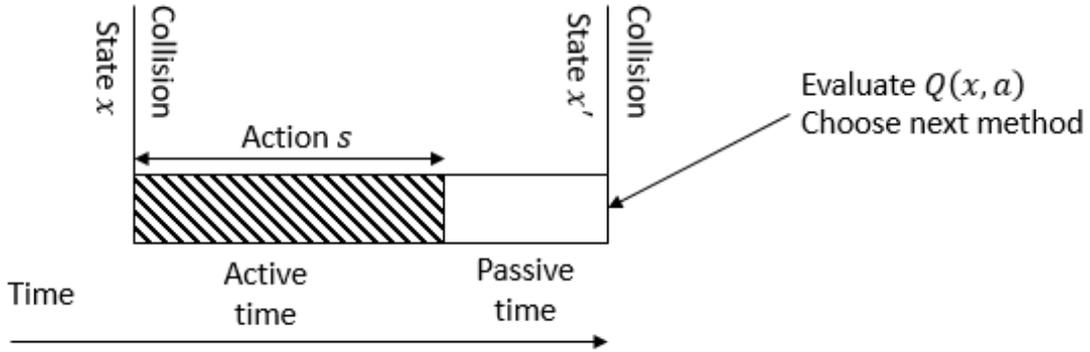
**Figure 3.3: Reactive arbitration using the Q-Learning algorithm.**
