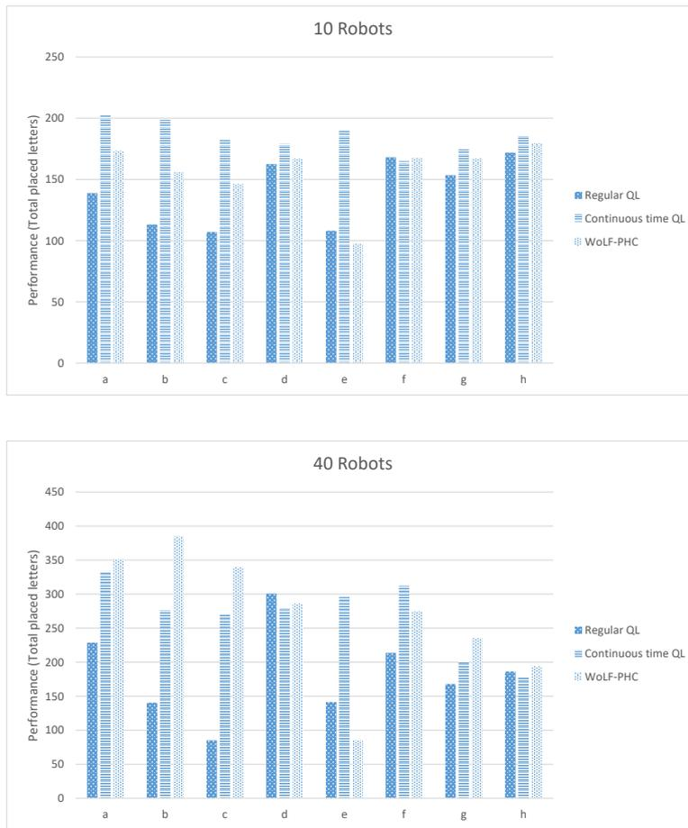
**Figure 5.18: Performance of the Minimum Over Actions approximation using action sets (a) to (h) with regular Q-Learning, continuous time Q-Learning and WoLF-PHC.**
