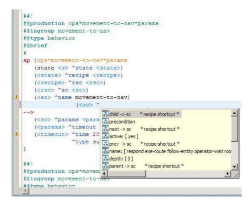
Figure 3.4: Auto complete with deep inspection
