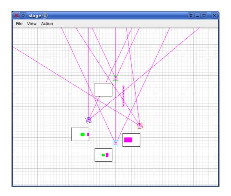
Figure 2.4: Robots running BITE'M in the player-stage API. The robots form a diamond. The lines mark visual field of view. Boxes with filled blocks show the colors perceived by each robot.
