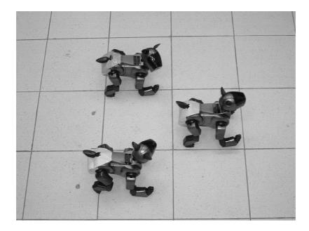
Figure 2.3: Sony AIBO robots moving in formation, controlled by BITE . Taken from [14, 15]
