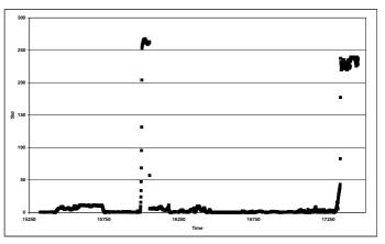
Fig. 3. Descend UAV C: Mahalanobis distance (in std units) as a function of flight time.
