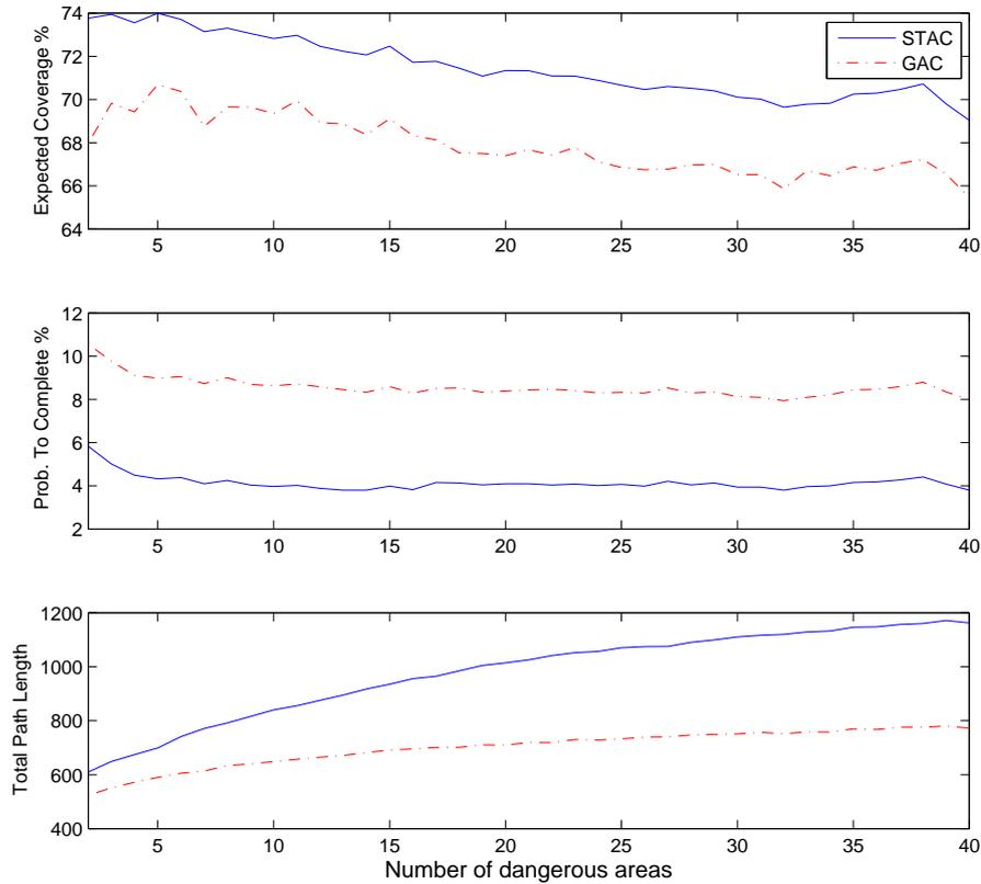
**Fig. 11.** Expected coverage percentage, probability to complete the coverage and total path length for different numbers of dangerous areas in environments with contiguous areas of threats.
