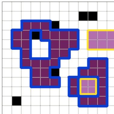
**Fig. 3.** An example of a grid containing two safe areas and five dangerous areas that belong to two different threat levels. The low-threat level areas are outlined by yellow lines and the high-threat level areas are outlined by blue lines.
