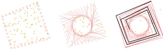
Fig. 3: The trails of the robots from their initial location (left) to their destination points in a straight movement (middle), and in a spiral movement (right). The black line emphasizes a trail of one specific robot.
