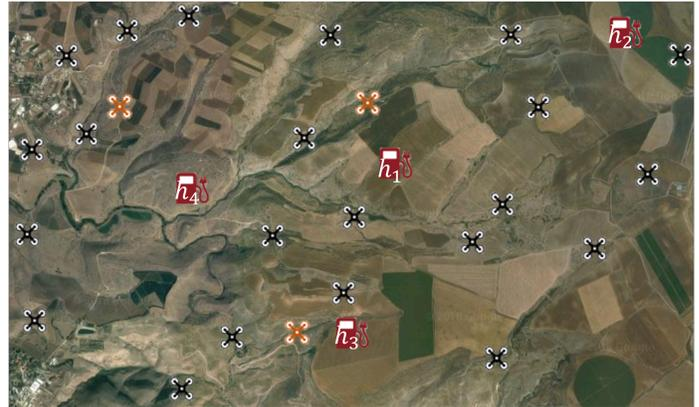
Fig. 1: Several locations requiring persistent monitoring, 4 charging/refueling stations ( $h_1, \dots, h_4$ ) and 3 spare drones (orange).
