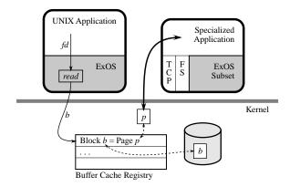
Figure 2-1: A simplified exokernel system with two applications, each linked with its own libOS and sharing pages through a buffer cache registry.
