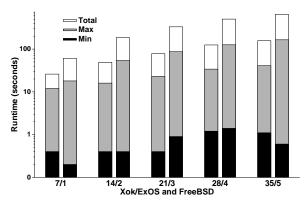
Figure 5-4: Measured global performance of Xok/ExOS (the first bar) and FreeBSD (the second bar), using the second application pool. Methodology and presentation are as described for Figure 5-3.
