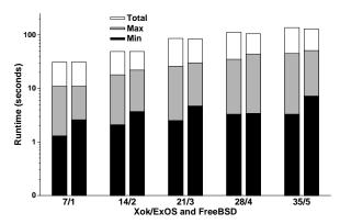
Figure 5-3: Measured global performance of Xok/ExOS (the first bar) and FreeBSD (the second bar), using the first application pool. Times are in seconds and on a log scale. *number/number* refers to the the total number of applications run by the script and the maximum number of jobs run concurrently. **Total** is the total running time of each experiment, **Max** is the longest runtime of any process in a given run (giving the worst latency). **Min** is the minimum.
