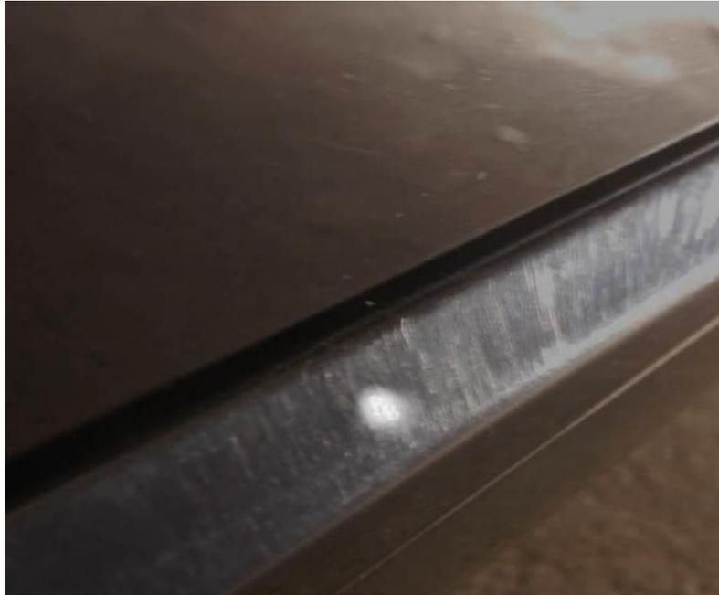
**Fig 5. Dirt on the tracks**
