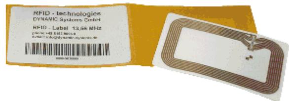
Fig. 1. Sticker of a RFID circuit and a bar code
