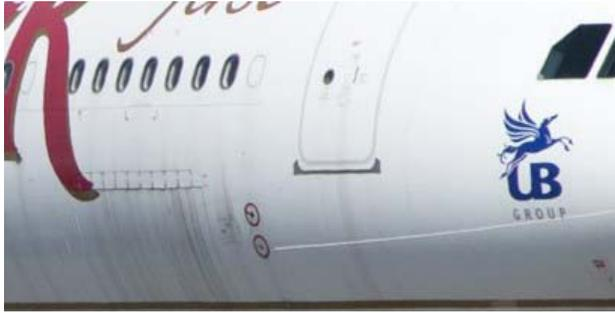
Figure 9. Dirt on the Fuselage
