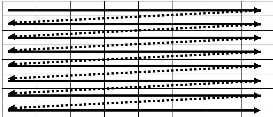
Figure. 2. The Order of the Lines in JPEG Image
