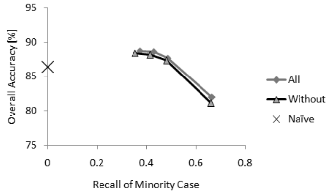
Figure 5: Comparing the overall model accuracy and recall for cases for disengaging the ACC
