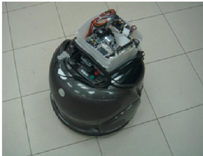
Figure 5.2: RV-400 robot used in initial experiments.
