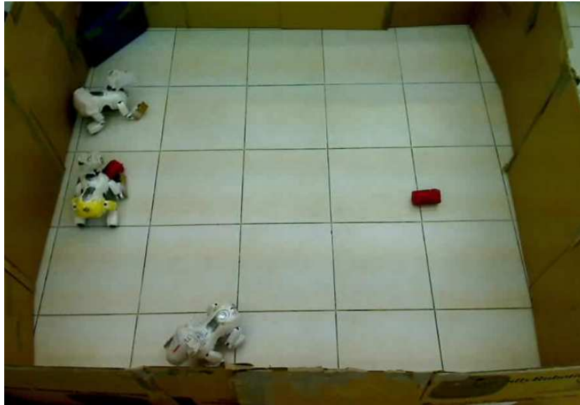
Figure 4.13: Three Sony AIBO robots executing a foraging task in our laboratory. The goal location is in the top left corner. Every puck collected was taken out of the arena.
