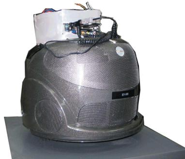
**Figure 2: The RV-400 vacuum cleaner robot, with our lab's computer overriding its commercial control software.**
