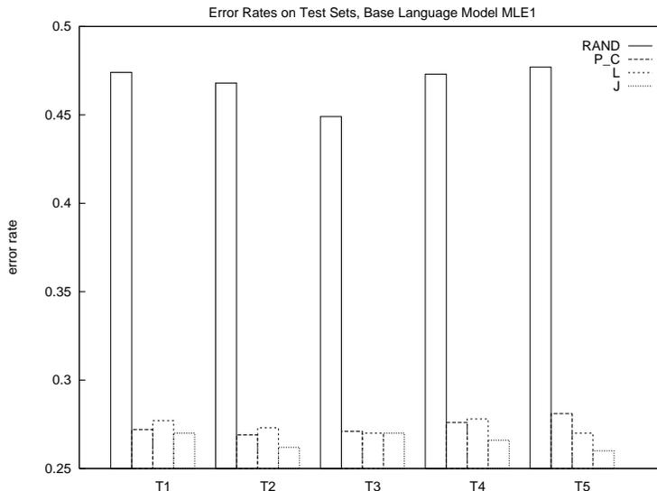
Figure 1. Error rates for each test set, where the base language model was MLE-1. The methods, going from left to right, are RAND,  $P_C$ ,  $L$ , and  $J$ . The performances shown are for settings of  $\beta$  that were optimal for the corresponding training set.  $\beta$  ranged from 4.0 to 4.5 for  $L$  and from 20 to 26 for  $J$ .
