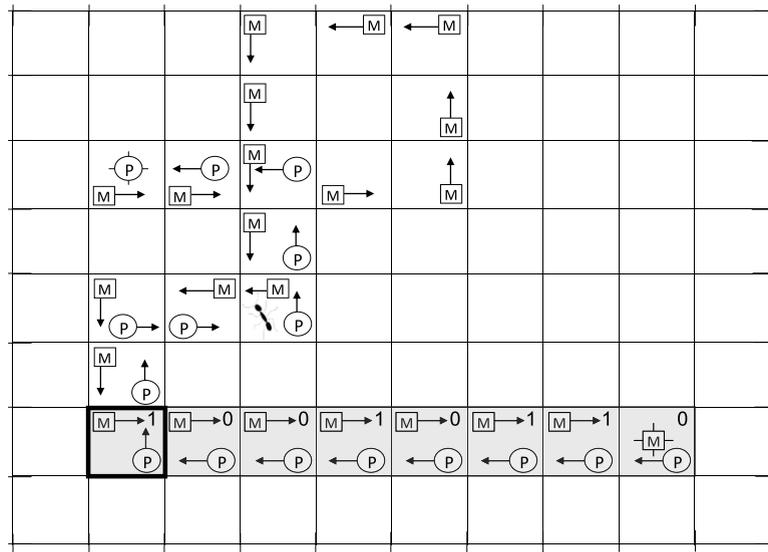
**Fig. 1.** An example of ElephantGun. The shaded region is the simulated Turing machine. *P* symbols are the *physical position* pointers. *M* symbols are the *memory position* pointers. The bold cell is the ant’s starting location.
