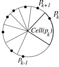
FIG. 6. Example of a circle division according to the Voronoi cells.
