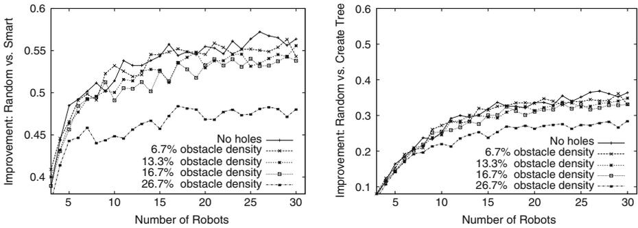
**Fig. 8** Comparison between the improvement ratio in coverage time obtained by algorithm NB\_MSTC (*left*) and Opt\_MSTC (*right*) after generating trees randomly vs. using Create\_Tree algorithm with different density of obstacles in the terrain
