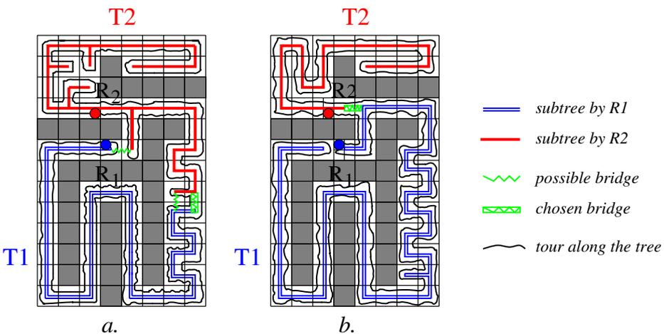
**Fig. 5** Illustrating the trees created using different distance measures by Procedure `Create_Tree`: **a** Manhattan distance and **b** Shortest paths
